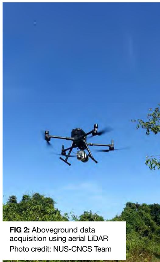
**FIG 2:** Aboveground data acquisition using aerial LiDAR
